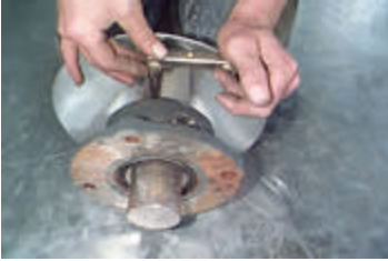
Photo 3. Tighten setscrews on metering drum bearing.
